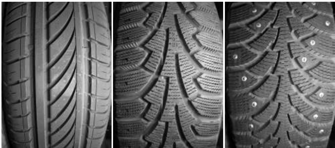
Figure 2. Tested tyre types. From left to right: summer, friction (non-studded winter) and studded tyres.
