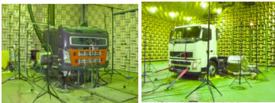
Figure 8.1 Powertrain rig (left) and Truck noise chamber (right) at the Noise and Vibration Laboratory, Volvo Trucks Göteborg
