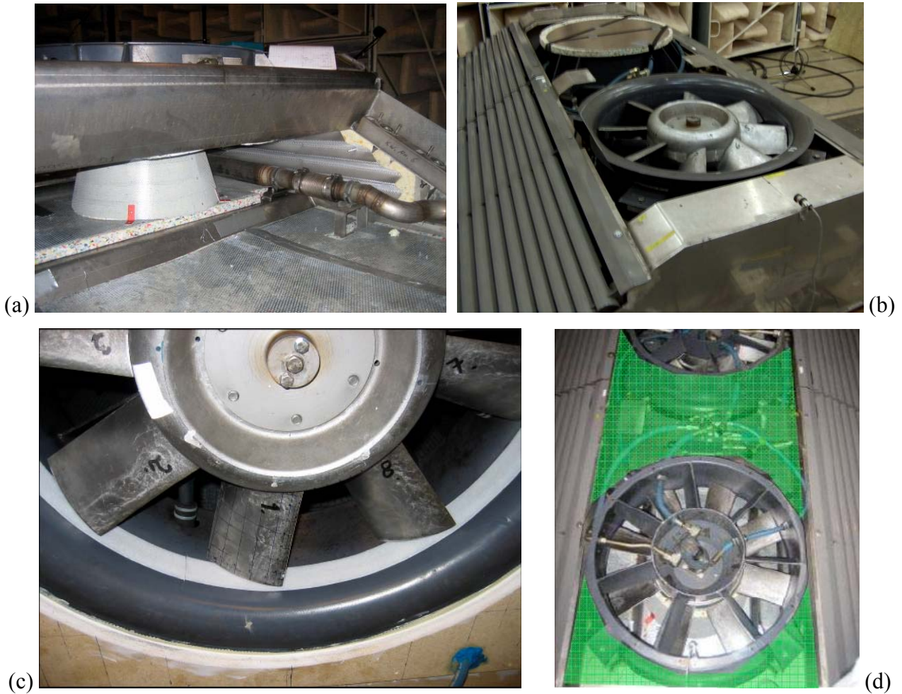
Figure 9: (a) Inside of cooling unit with interior absorption and flow guide cones. (b) Upper side of cooling unit with one fan mounted in reversed mode. The other fan is deactivated and sealed off. (c) Velcro tape on stator circumference, (d) Shaded area shows where outside absorption was placed.
