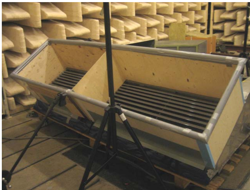
Figure 8: Box used for measurements of inlet/outlet flow velocity by hand held scanning hot wire probe.
