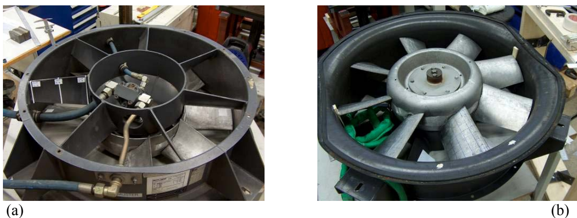
Figure 2: (a) Inlet side of fan, (b) Outlet side of fan. The hydraulic engine with seven pistons is visible inside the hub.
